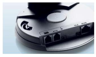
**Easy set up** The GN 9330 base could not be simpler to setup. An easy-to-operate slide control facilitates dial tone adjustment. After securing a clear, audible dial tone the microphone volume wheel can be used to set the transmit volume of your voice, ensuring that the conversation will be heard properly at both ends of the line.
